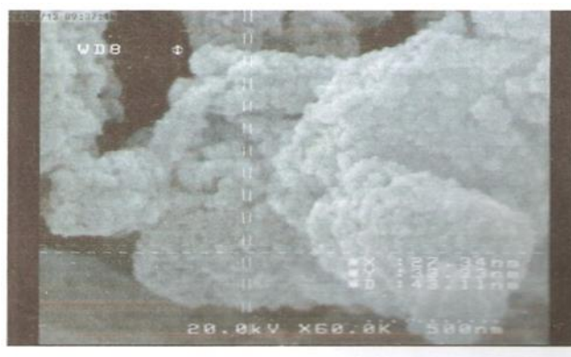
Figure 3. The SEM image of nanosilica particles supported by sodium hydrogen sulfate
