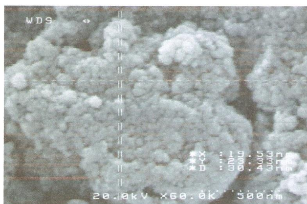
Figure 2. The SEM image of nanosilica particles
